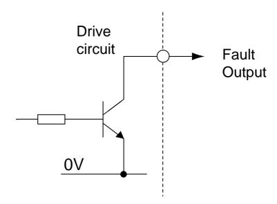
Figure 3-16. Fault Output Circuit
